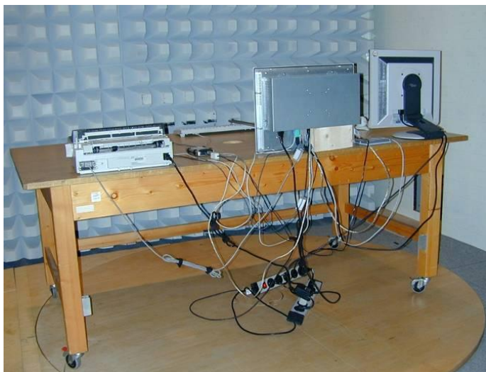
Picture 5 EMC: Test setup for CE conformity verification
