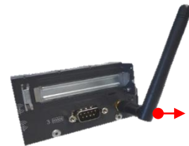
WLAN antenna installed (customer option)
